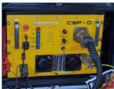
c) CSP-D2000 capacitor bank
