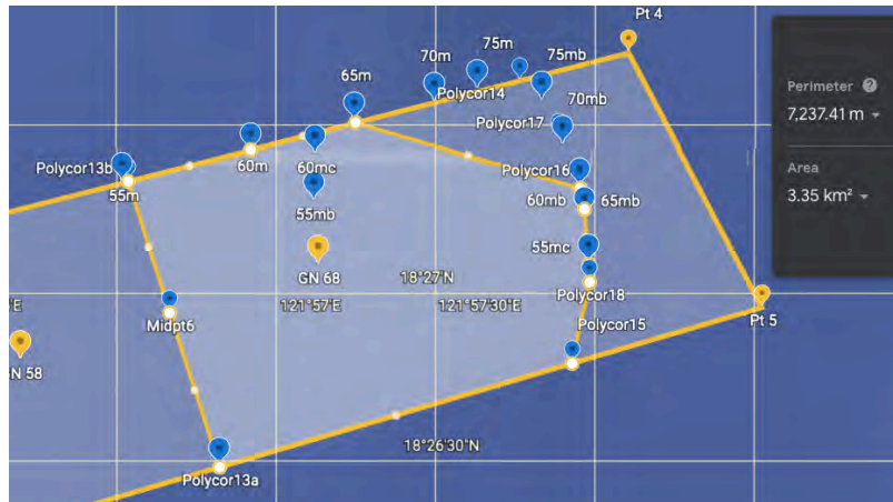
Figure 22. Polygon construction at GN 68 at Level -65m.
