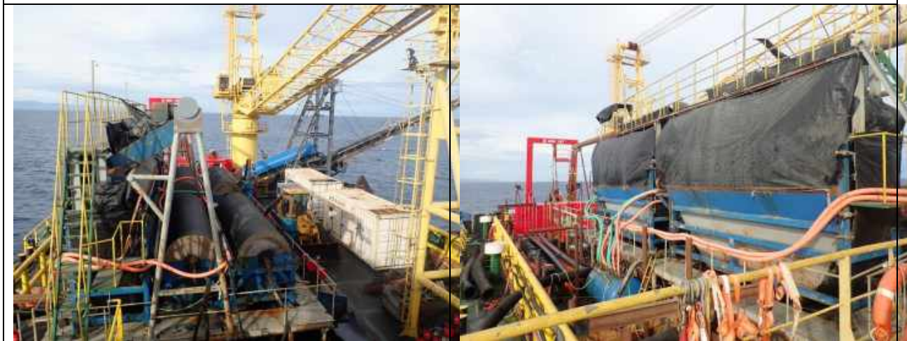
Photo 6. Operation set-up for magnetite extraction
