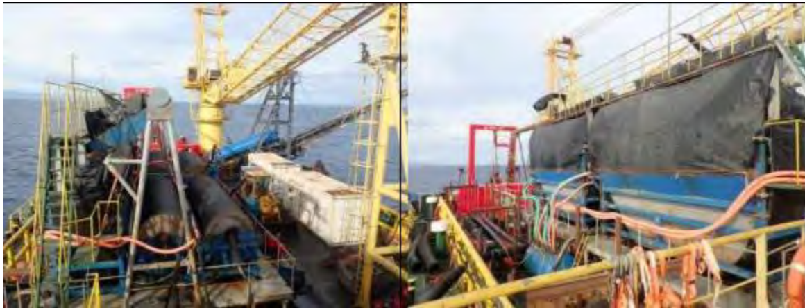
Photo 7. Operation set-up for magnetite extraction (left) 3-stage magnetic separator system (right)
