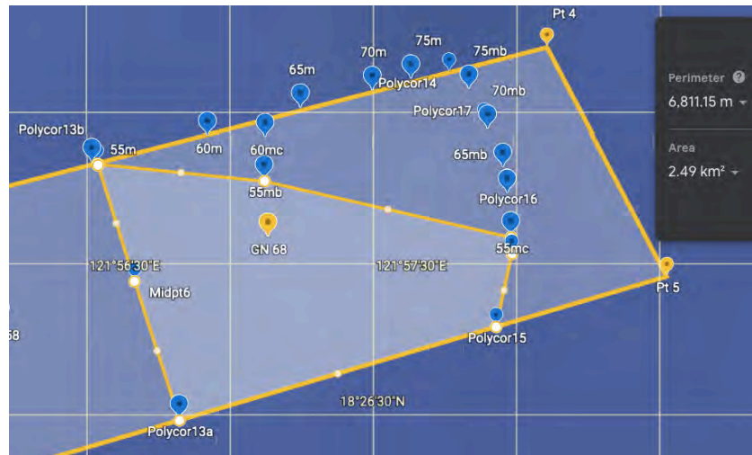
Figure 20. Polygon construction at GN 68 at Level -55m.
