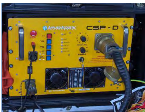
c) CSP-D2000 capacitor bank
