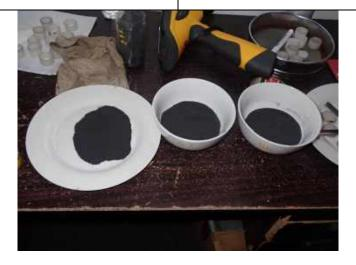
**Photo10**. Samples of magnetite sand after processing.
