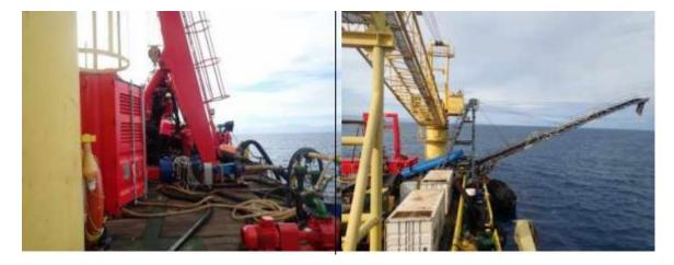
Photo 8. Extraction/siphon pump (left); Flyout conveyor where waste materials will go back to the sea
