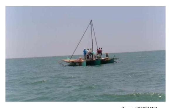
Source: JDVCRC FER **Photo 1.** A Longyear 38 Rotary Drill mounted in 3 interconnected boats
