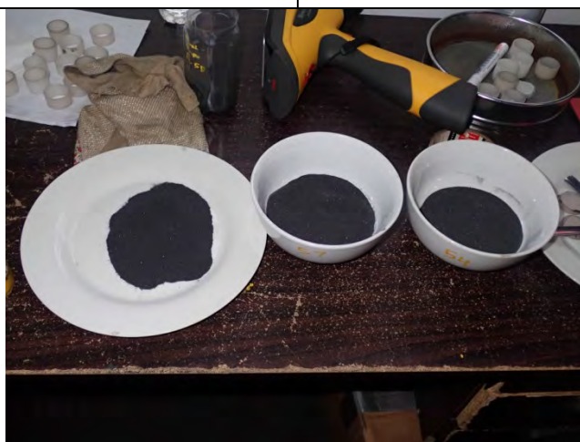
Photo10. Samples of magnetite sand after processing.
