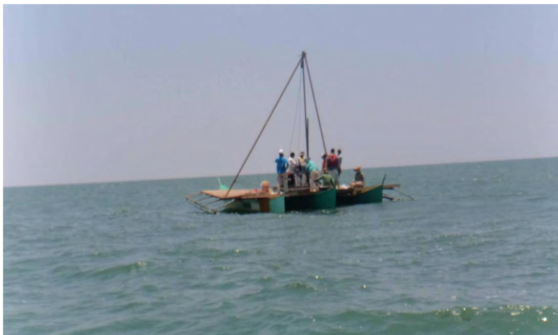
Photo 1. A Longyear 38 Rotary Drill mounted in 3 interconnected boats
