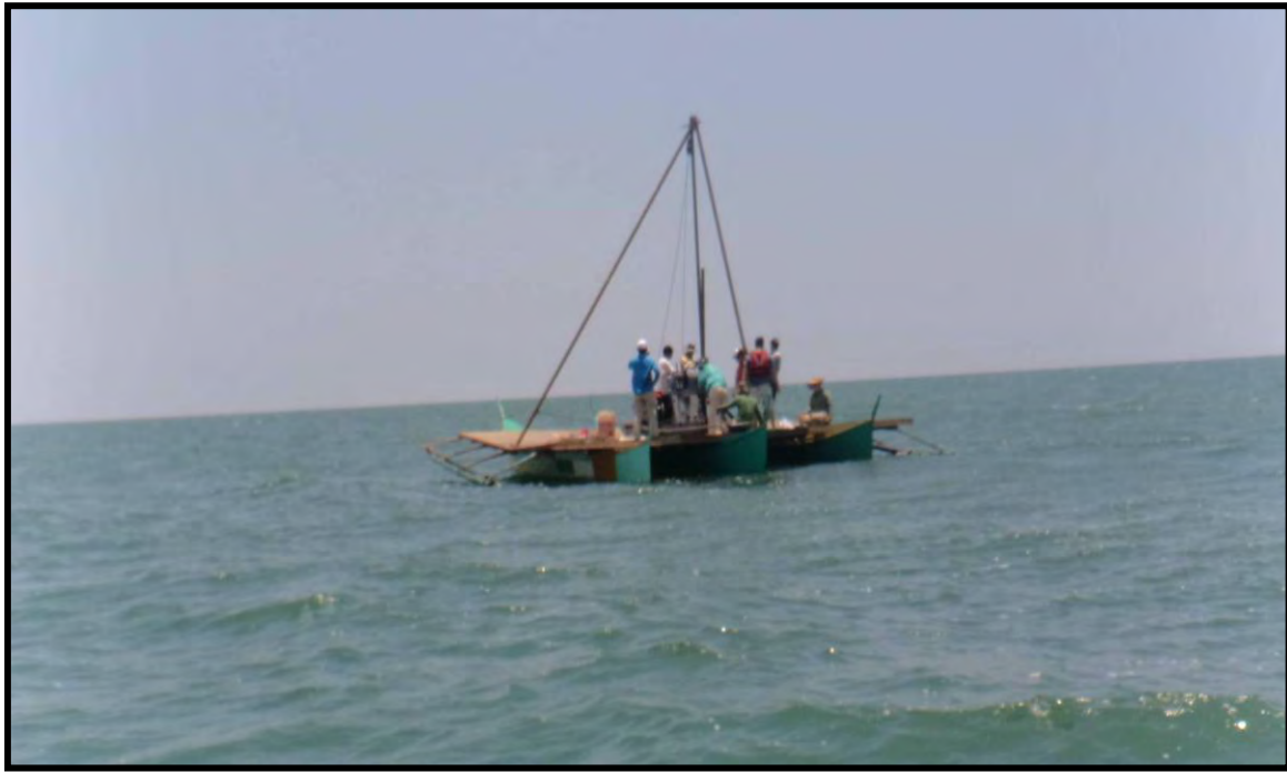
Figure 14.3.1.1: A Longyear 38 Rotary Drill mounted in 3 interconnected boats
