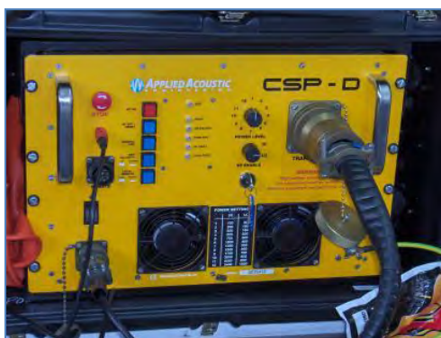
c) CSP-D2000 capacitor bank
