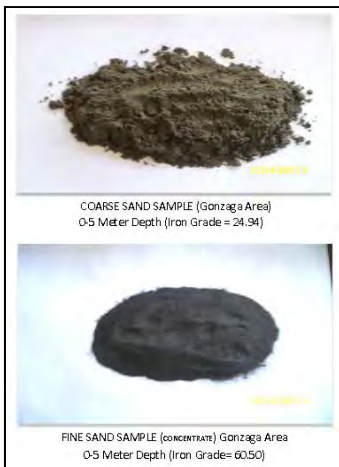
Figure 13.8.1: Pictures Showing the Raw Sand and Magnetite Concentrate Samples
